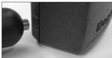
Figure 7: Using the test light magnet to reset the R8 Receiver
